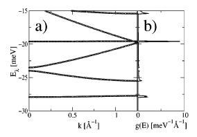
FIG. 1. (a) Calculated band structure of a <sup>4</sup>He atom adsorbed in the interstitial channel. (b) The corresponding density of states per unit length.
