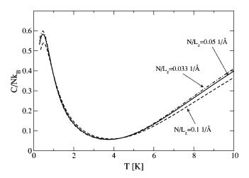
FIG. 3. Isosteric specific heat of  $^4$ He gas within the nanotube interstitial channels as a function of the sample temperature for three different average He linear densities  $N/L_z$ . Dash-dotted line:  $N/L_z = 0.033\,$  1/Å. Full line:  $N/L_z = 0.05\,$  1/Å. Dashed line:  $N/L_z = 0.1\,$  1/Å
