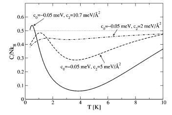
FIG. 4. Dependence of specific heat of  $^4{\rm He}$  gas on the corrugation of the interaction potential along the channel axis. Full line:  $c_0\!=\!-0.05$  meV,  $c_2\!=\!10.7$  meV/Å $^2$ . Dashed line:  $c_0\!=\!-0.05$  meV,  $c_2\!=\!5$  meV/Å $^2$ . Dash-dotted line:  $c_0$ =-0.05 meV,  $c_2\!=\!2$  meV/Å $^2$ . In these calculations, the average linear density of  $^4{\rm He}$  atoms was set to 0.1 1/Å.
